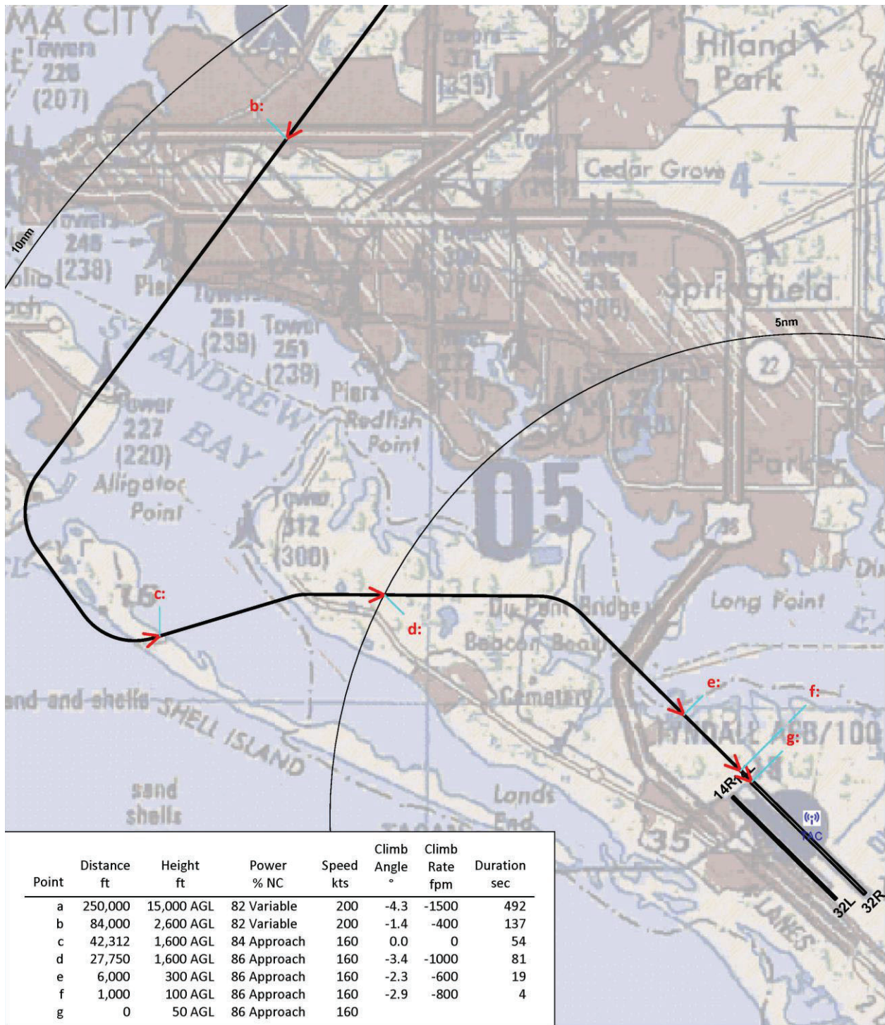
Flight Profile ADLA09 ADAIR LOW NOISE VFR FROM COMPASS LAKE Flight Track: 4LA1CL - 14L base to final from Compass Lake Aircraft: ADAIR Cat C Low Engine: F100-PW-100 Scale in Feet 1:78,400 (1 inch = 6,530 feet)
